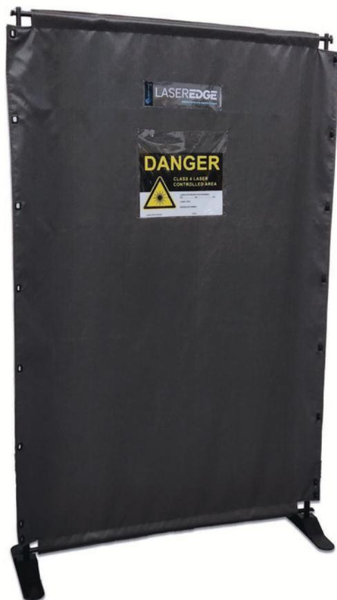
The LaserEdge PLUS is a laser safety barrier that protects  $425\text{W}/\text{cm}^2$  for at least 100 seconds, wavelength 1070nm, 1mm diameter spot (1/e). With a lightweight design, this laser safety barrier has the exclusive LaserEdge technology, with a single panel and integrated light-blocking strip.
