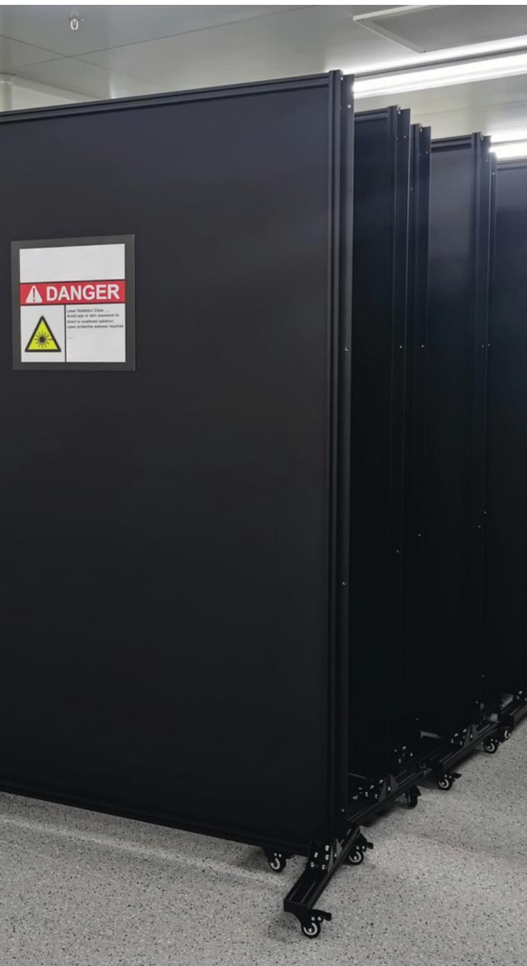
Laser barriers are an important part of laser safety measures, and their proper use and maintenance are crucial to avoid accidents or injuries caused by laser radiation. As such, it is important that they meet or exceed the safety standards set by the American National Standards Institute (ANSI) 136.1, as is the case with the barriers available at Phillips Safety. This certification ensures that all of our laser barriers provide the necessary protection for safe use of lasers.
