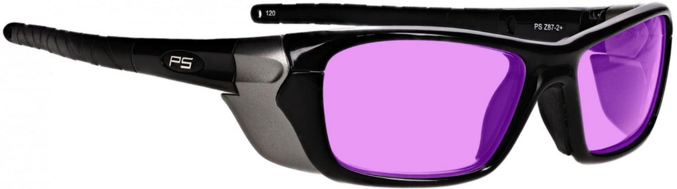
The lampworking glasses Phillips 202 have a glass violet lampworking lens that provides excellent color recognition for soft glass. These frameworking glasses offer excellent UV blocker, good IR protection, excellent sodium flare blocker, and excellent clarity. Recommended for those who work with lampwork or hot glass in small pieces.
