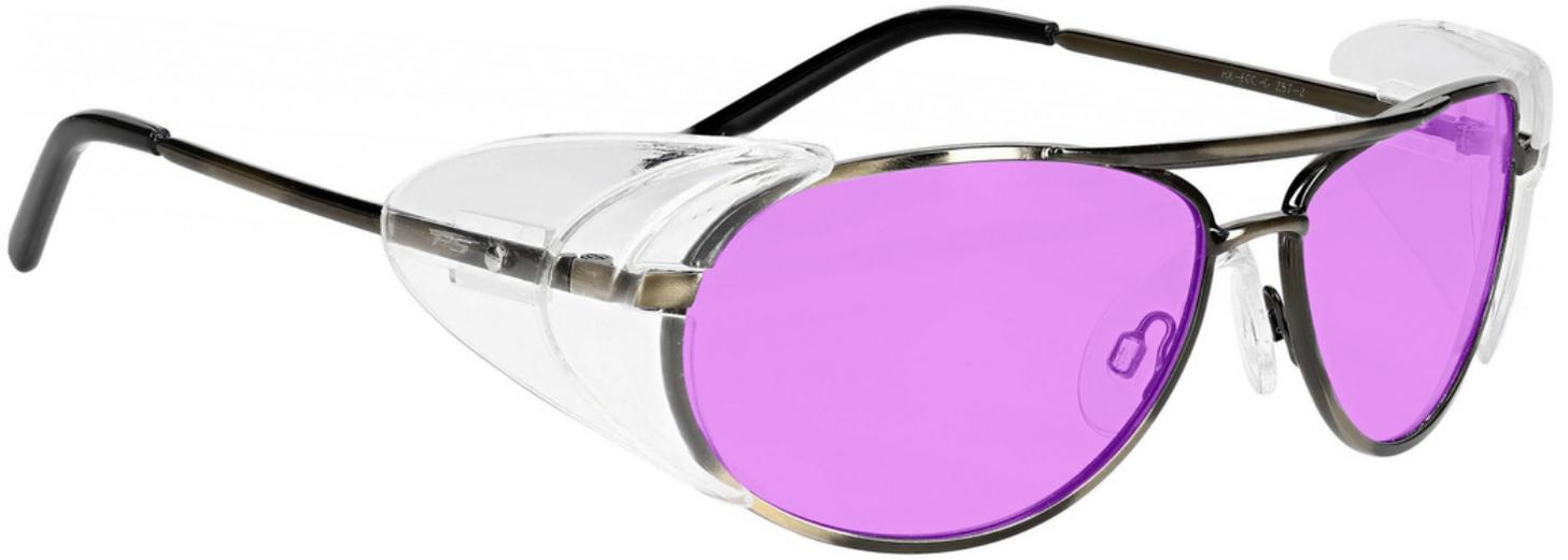
The lampworking glasses Phillips 202 have a glass violet lampworking lens that provides excellent color recognition for soft glass. These frameworking glasses offer excellent UV blocker, good IR protection, excellent sodium flare blocker, and excellent clarity. Recommended for those who work with lampwork or hot glass in small pieces.
