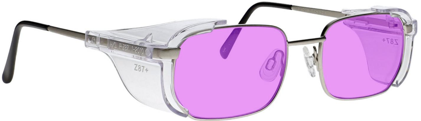
The lampworking glasses Phillips 202 have a glass violet lampworking lens that provides excellent color recognition for soft glass. These frameworking glasses offer excellent UV blocker, good IR protection, excellent sodium flare blocker, and excellent clarity. Recommended for those who work with lampwork or hot glass in small pieces.
