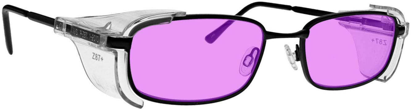
The lampworking glasses Phillips 202 have a glass violet lampworking lens that provides excellent color recognition for soft glass. These frameworking glasses offer excellent UV blocker, good IR protection, excellent sodium flare blocker, and excellent clarity. Recommended for those who work with lampwork or hot glass in small pieces.
